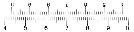
other to the focusing ring, it is possible to estimate the focus position to 1/10th of the smallest division of the longer scale. To do this you simply look at where the left index mark on the left of the short scale falls on the longer scale. Suppose it lies between 6.5 and 6.6 as shown in the image below. Then you look for which of the short division marks lines up with those of the longer scale. Suppose it is the 5th one. Then the scale
