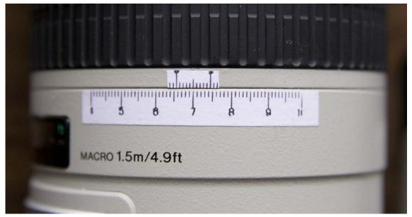
reading is 6.55. A magnifier can be used if needed and of course, a red flashlight is required in the dark.
