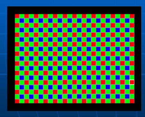
Sensors can be made colour sensitive by applying a colour mosaic to the sensor
